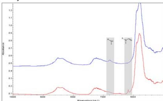
Figure 2. NIR spectra at the start (blue) and the end (red) of the reaction.
